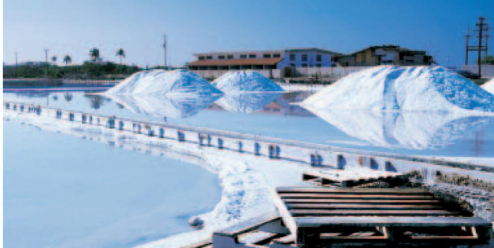
**Figure 13** This ocean-salt recovery site uses evaporation to separate the halogen compounds from the water so the salts can be refined further.
