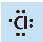
Figure 13 Electron dot diagrams show the electrons in an element's outer energy level.
