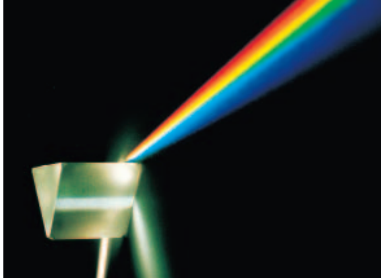
Figure 6 Refraction causes a prism to separate a beam of white light into different colors.
