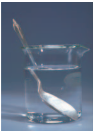
Figure 5 The spoon looks bent because light waves are refracted as they change speed when they pass from the water to the air.
