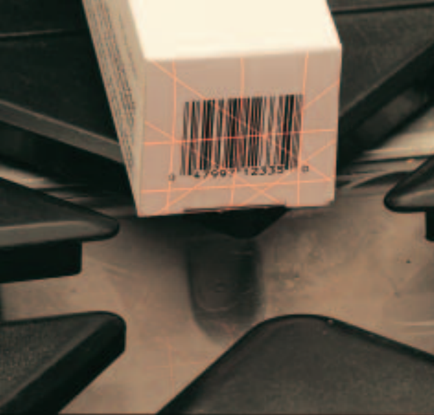
Figure 25 Optical scanners like this one use lasers to find the price of various products.
