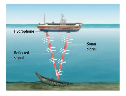
underwater sound waves to detect objects. First, a sound pulse is emitted toward the bottom of the ocean. The sound travels through the water and is reflected when it hits something solid, as shown in **Figure 20.** A sensitive underwater microphone called a hydrophone picks up the reflected signal. Because the speed of sound in water is known, the distance to the object can be calculated by measuring how much time passes between emitting the sound pulse and receiving the reflected signal.
