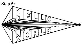
Decide the depth of the letters and use the vanishing points to create a guide for where that back edges of the letters should be placed.
